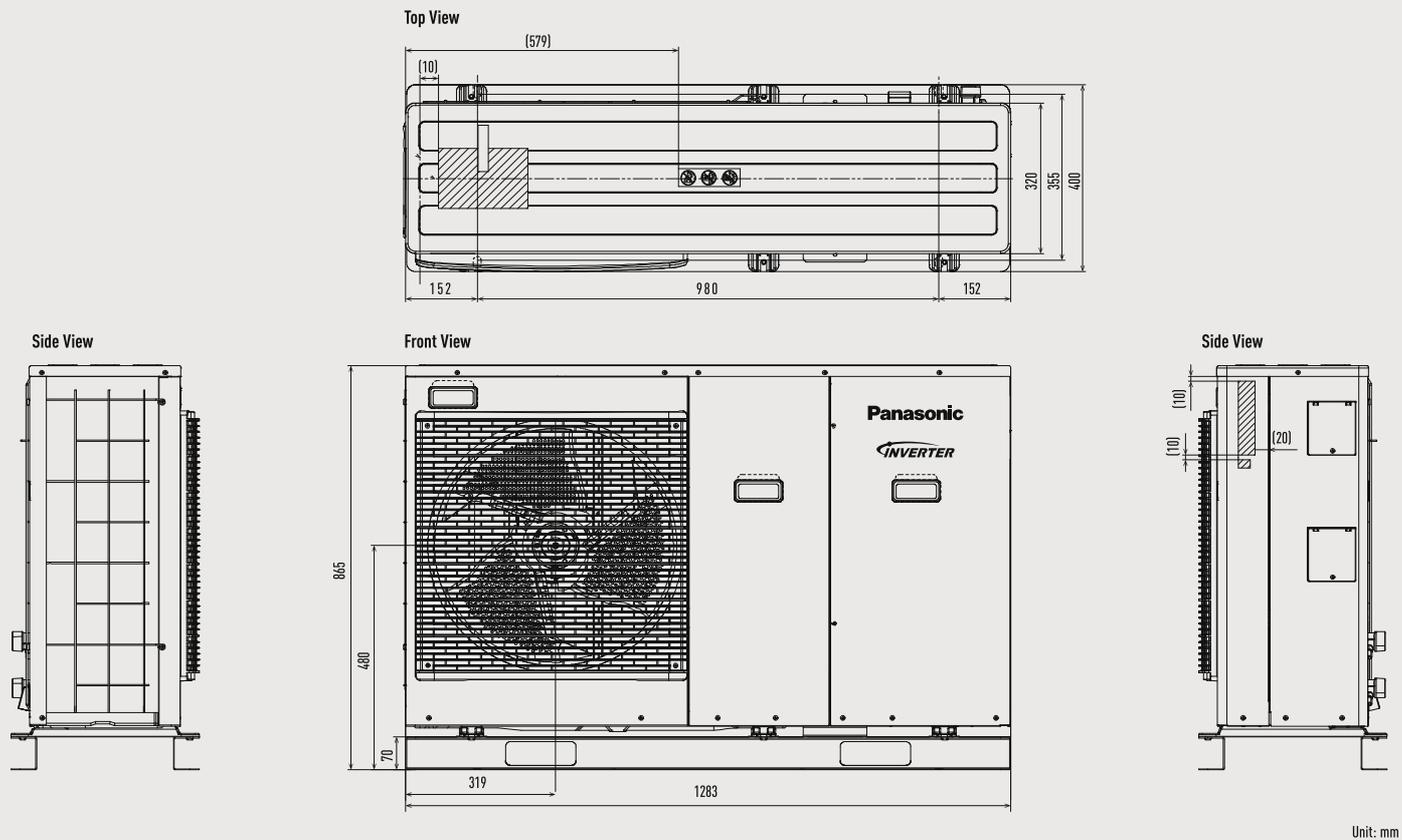
Bi-bloc Super Quiet outdoor unit and Mono-bloc outdoor unit from 9 to 16kW
